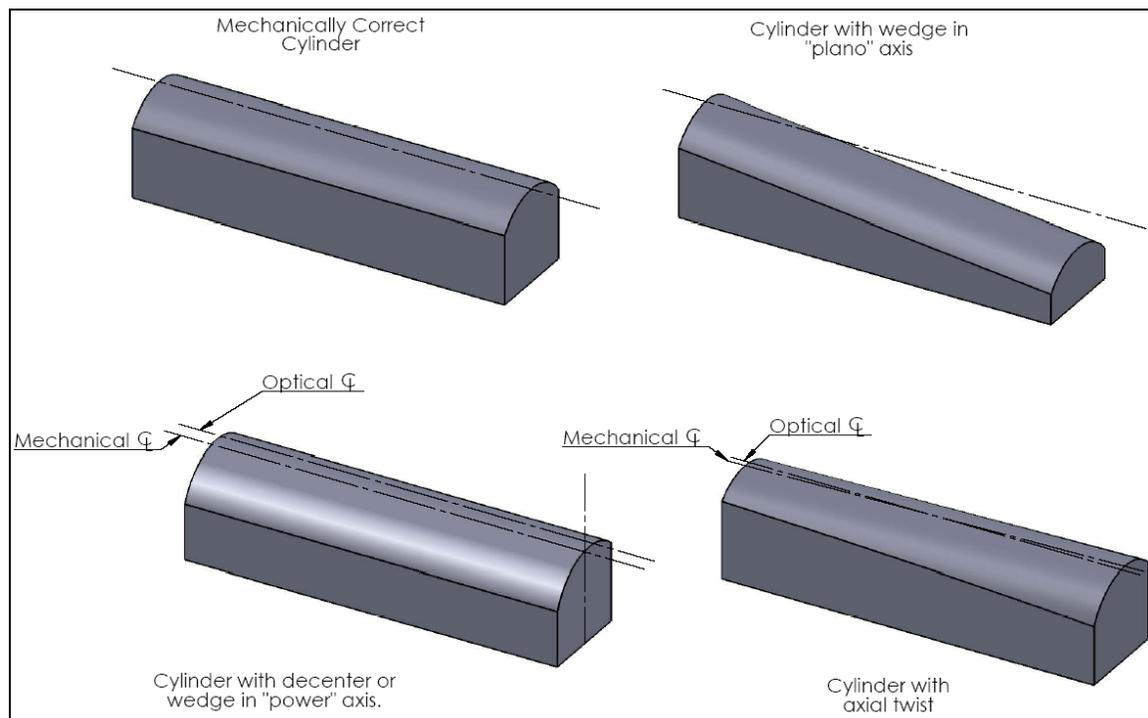
Figure 1 - Representations of centration errors for cylindrical lenses
