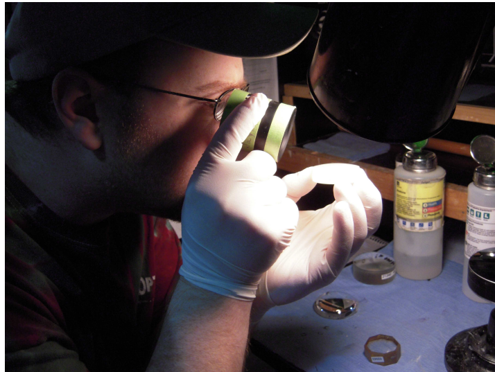
Figure 3 – Visual surface inspection of ZnS surface
