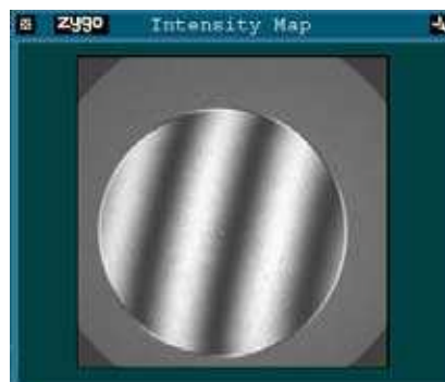
Figure 2: TWE map showing TWE is < \lambda/30 .
