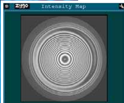
Figure 1: Image of an error-laden reflected wavefront of one surface of an asphere.
