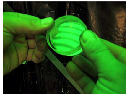
Figure 5: Test Plate Fringe Pattern
