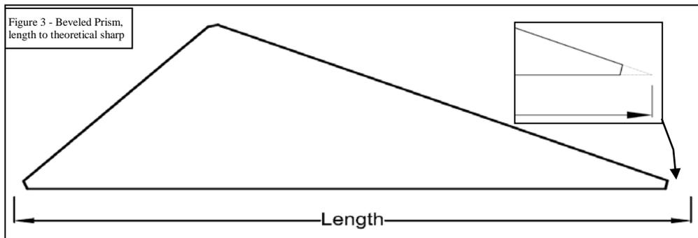
Figure 3 - Beveled Prism, length to theoretical sharp
