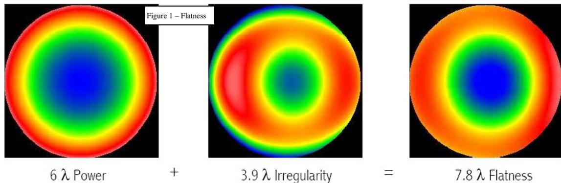
Flatness is typically measured in double-pass using a reflected wavefront, where the magnitude of the wavefront error is twice the flatness. Fringe analysis software accounts for the double-pass, dividing the value for the user<sup>1</sup>.
