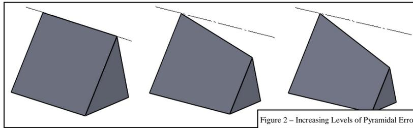
Figure 2 – Increasing Levels of Pyramidal Error
