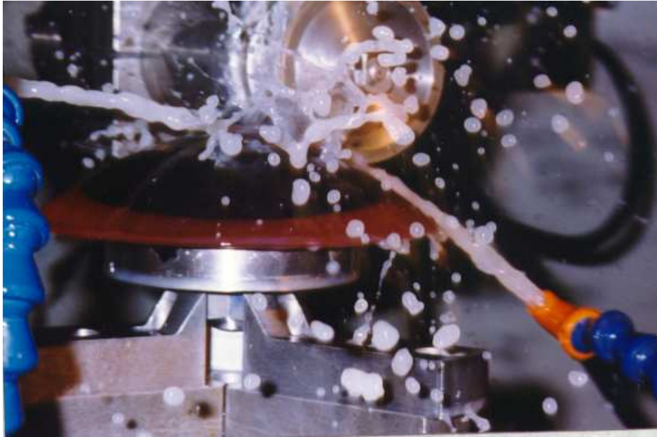
<<Figure #9: Precision Fabrication of Aspheric Lenses via CNC Machining >>
