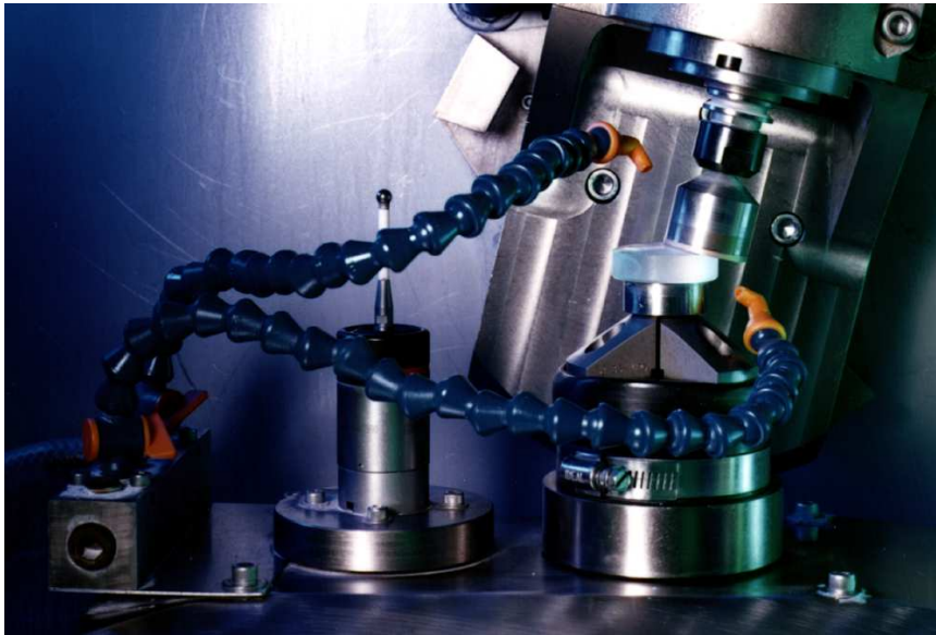
<<Figure #7: Deterministic Grinding with CNC Machine>>
